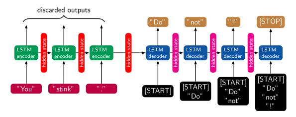
Recall that the words are first all tokenized, and the output of the decoder is fed back into itself. Only the encoder's *final* hidden state is passed to the decoder.
