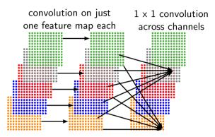
Xception networks are built out of this module, combined with max-pooling layers.
