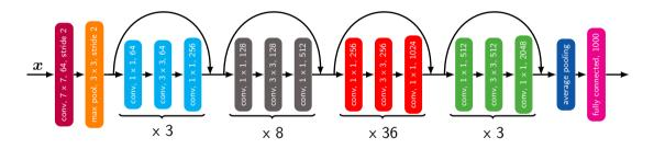
Rather than bypass just 2 layers, ResNet 152 is built out of blocks which bypass 3 layers. The winner of ILSVRC 2015. 152 layers!
