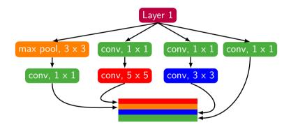
$1 \times 1$  convolutional layers are used to reduce the dimensionality of the input, making the computation more manageable.
