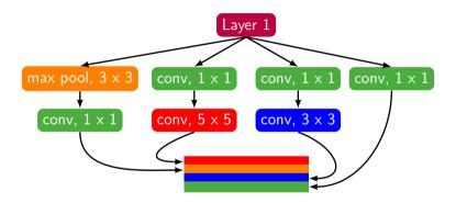
$1 \times 1$  convolutional layers are used to reduce the dimensionality of the input, making the computation more manageable.
