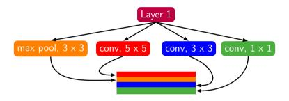
The outputs of the layers are bundled into a single input for the next layer.
