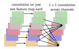
Xception networks are built out of this module, combined with max-pooling layers.
