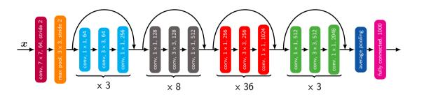
Rather than bypass just 2 layers, ResNet 152 is built out of blocks which bypass 3 layers.
