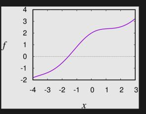
Algorithms always start from an initial guess and (usually) a bounding interval [a, b] in which the root is to be found.
