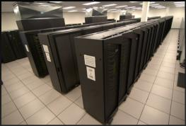
Number of nodes: 42 interconnect: Infiniband RAM/node: 64 GB Cores/node: 16 Niagara
