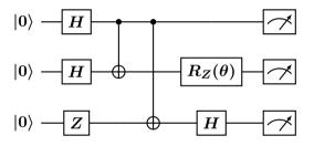
Time runs from left to right. Each "wire" in the circuit represents a qubit. The various gates and operations are represented by boxes or connections between the wires. The rightmost symbol is a measurement.
