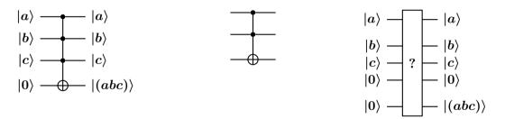
The auxiliary qubit should both start and end in the  $|0\rangle$  state. The PennyLane Toffoli function takes a list of 3 wires as its argument. The first two wires are the control, the third is the target.
